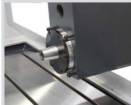
Our tested guarantee of spindle run out is up to 0.0015 mm. The high precision preloaded roller thrust and radial bearings ensure minimum spindle runout. A special lubricant and extremely high-quality bearing seals provide a long-term durability.
