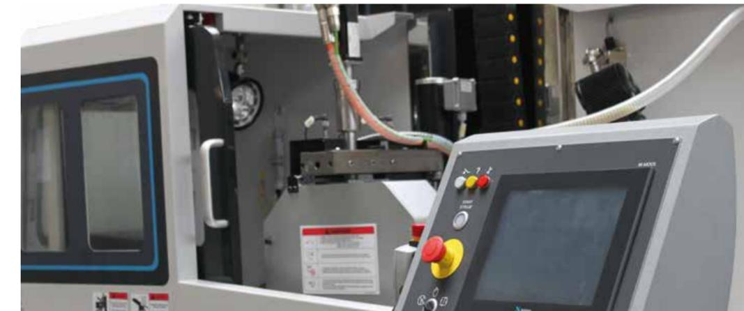
10" touch screen and ergonomically placement of control elements ensure Easy and Fast operation
