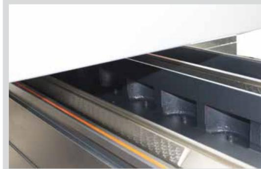
The main feature are hand scraped V-V guideways in longitudinal and cross axis. This type of guideway perfectly absorbs vibrations and provides a high linear accuracy. Length of guideways surfaces are proportional to the length of travel worktable so there is no twisting or floating of workbench.
