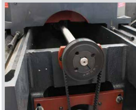
Standard machine version used servomotors for driven cross and vertical axis. The each axis is equipped with precision ball screws of Czech manufacturer KSK, which provide a long-term working accuracy.
