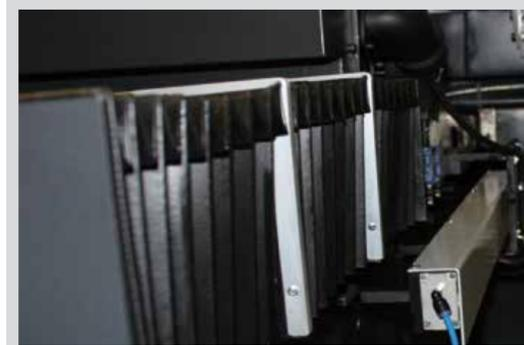
Cross and vertical axis is fitted by linear scales ESSA Prague with an accuracy of 0.001 mm, which ensures high positioning accuracy. Dust protection of scale is ensured by supply of compressed air directly into the scale. The air is perfectly filtered through HEIDENHAIN DA 400, which provides filtration of particles less than 0.01 micron.
